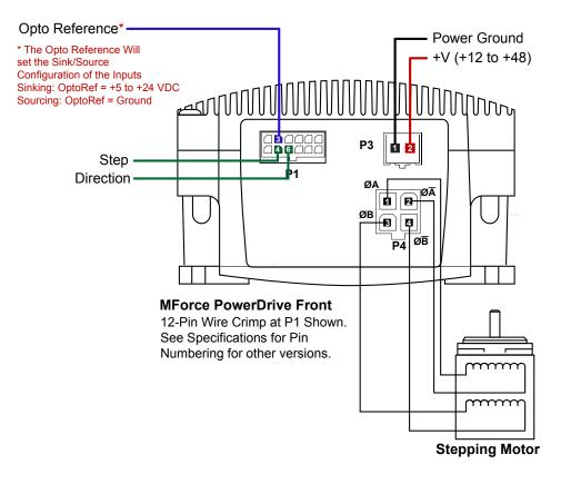
Figure 2.4.7: Minimum Required Connections
